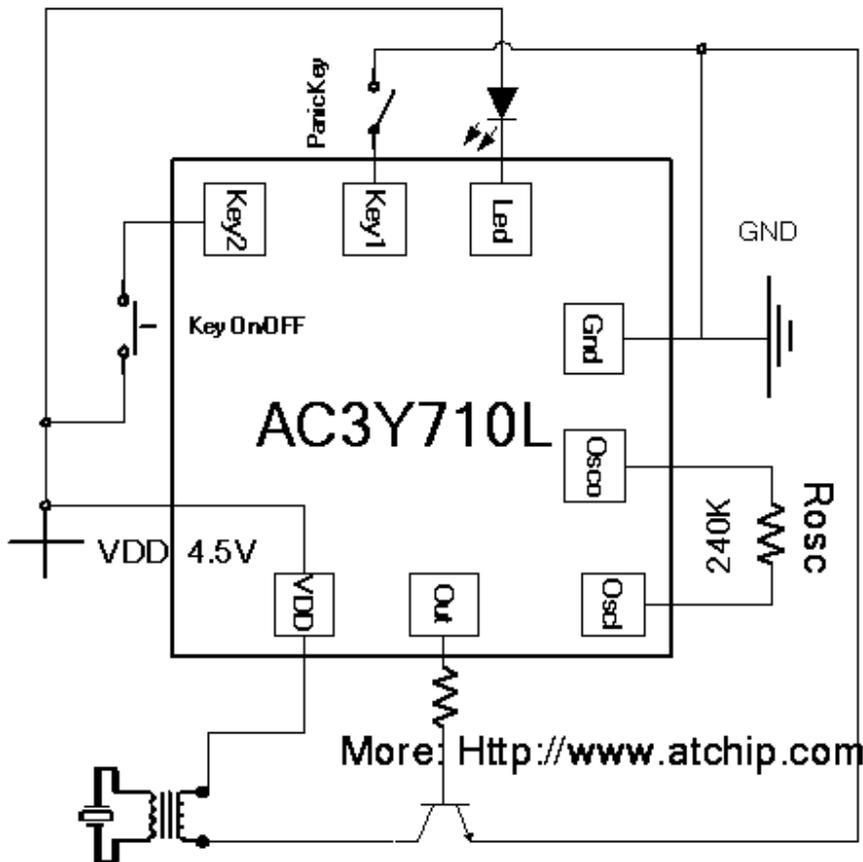
**THE IC SUBSTRATE SHOULD BE CONNECTED TO VDD**
